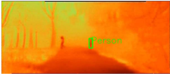
Figure 11. Results of detection of a group of people (2 persons) on images recorded with a telephoto lens on fog, 50m distance, using bYOLO (a) opposite to tYOLO model (b).
