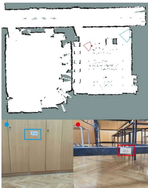
Fig. 6. Example of labels used for search and rescue task and their location on the map (marked in red and blue along with their locations on the map)
