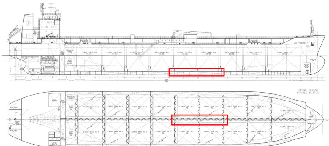
Figure 11. General arrangement of the Panamax tanker and damage extent.
